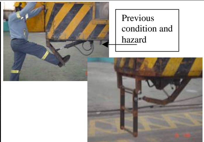
Figure 2.- This modification keeps stair fixed even without power or air supply fail.
