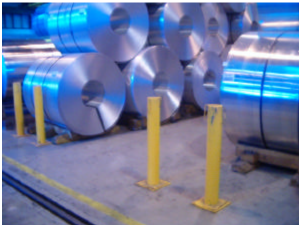
Figure.3 Steel bars were mounted both end of the Storage lines of the coils.
