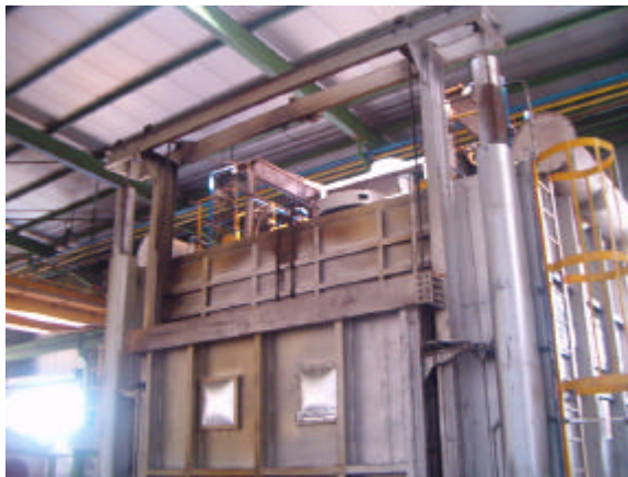
Figure 1. Annealing furnace without safety locking.
