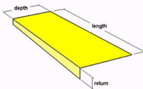
Stair covers usually are constructed from a durable, high impact polyester or steel plate and feature a diamond hard silicon carbide aggregate anti-slip surface.
