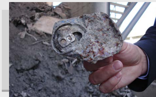
Pictures of molten cans and aluminium recovered from bottom ashes
