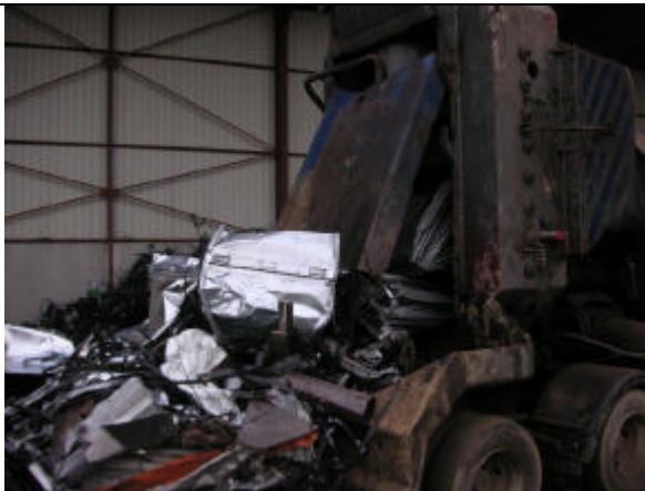
Figure 31. A shearer in use at a local metal trader in Troyes, France. Such machines are used to prepare large parts of Aluminium extracted from CVs.
