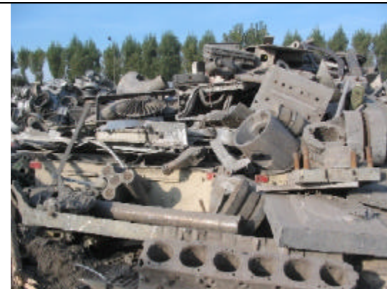
Figure 36. Aluminium-concentrated parts coming from public works equipment at an aluminium preparation plant in Paris region, France.
