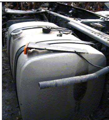
Figure 23. One aluminium tank extracted from an injured CV, here in Roncq, France.
