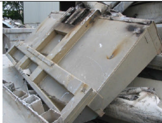
Figure 26. Detail view of some aluminium parts (a tipper body) extracted from EoL commercial road vehicles at a local metal dealer in Troyes, France.
