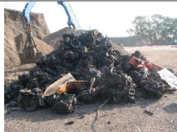
Figure 34. Foundry part as input of an aluminium preparation plant in Paris region, France.
