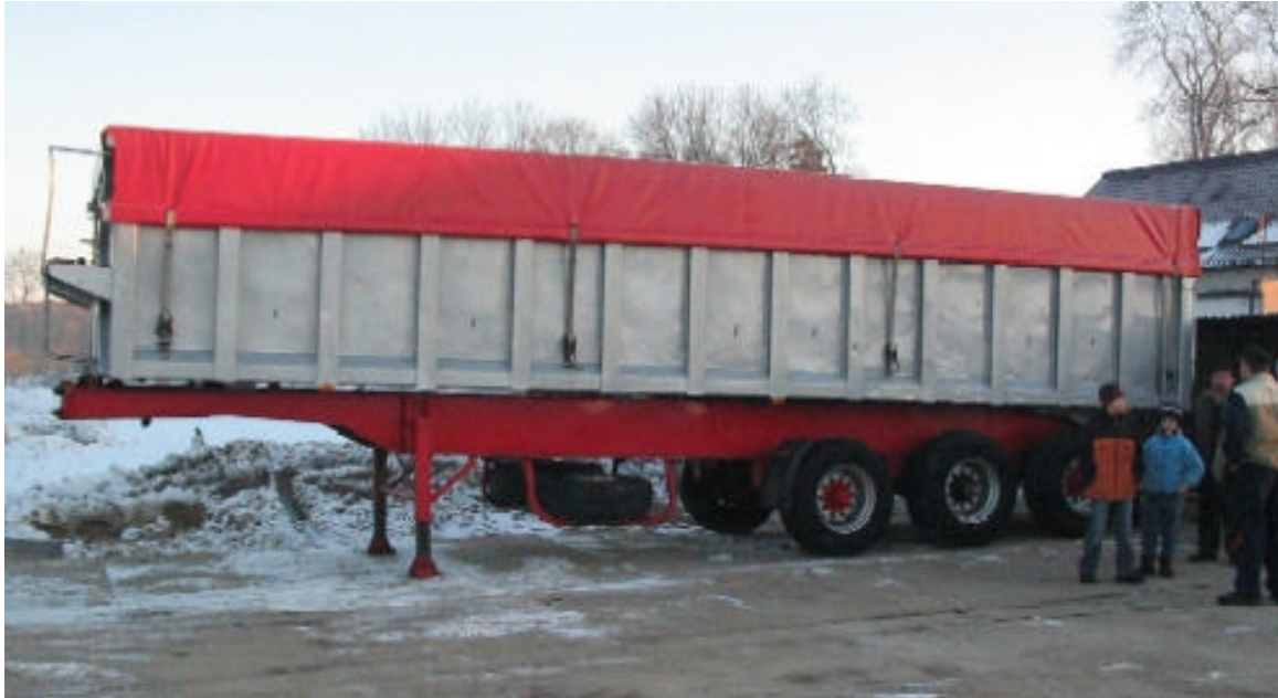
Figure 17. A 1988 Ova trailer in use at a small transport company in the North of Poland. The tipping body is made of aluminium while the chassis is made of steel.
