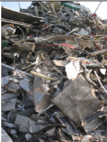
Figure 33. Laminated parts as input of an aluminium preparation plant in Paris region, France. It was observed that this flow contains some parts coming from CV.
