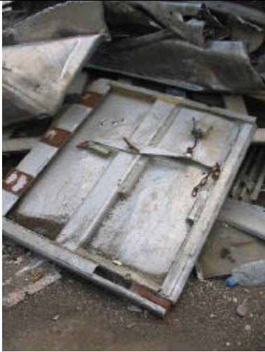
Figure 29. Detail view of some aluminium parts (a door) extracted from EoL commercial road vehicles at a local metal dealer in Troyes, France.
