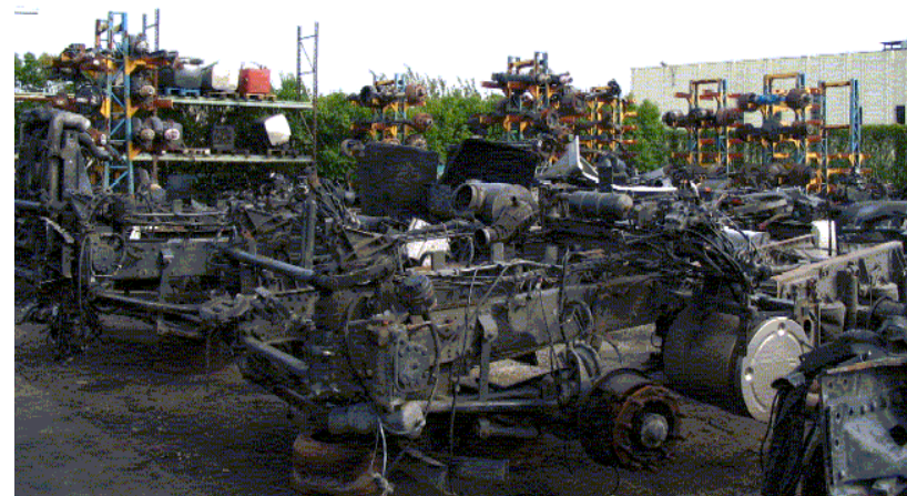
Figure 24. Bodies of injured CV after the extraction of all valuable parts; the body is ready to be sent to the local shredder; here in Roncq, France.
