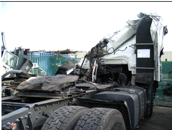
Figure 21. An injured MCV as it can be received at a dismantling plant, here in Roncq, France.
