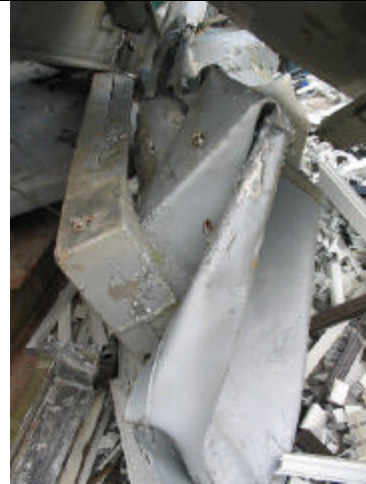
Figure 30. Detail view of some aluminium parts (a tipper body) extracted from EoL commercial road vehicles at a metal dealer in Troyes, France.
