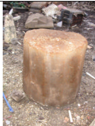
Figure 32. A "ball" used in many local metal dealer to liberate metals in parts like motors, gear boxes, etc.
