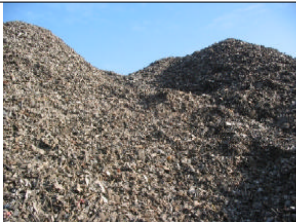
Figure 35. Aluminium concentrated fraction coming from shredders, in Paris region, France.
