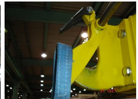
Automatic unhooking of belts from the traverse
