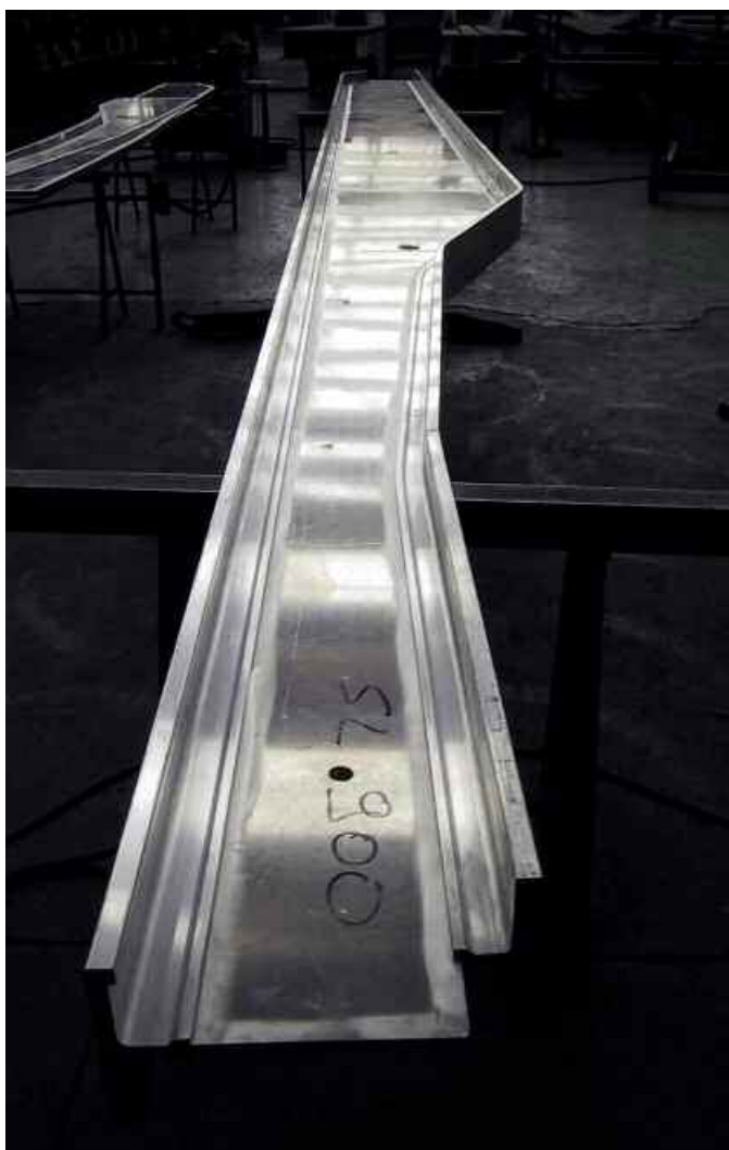
Semi-trailer chassis beam made out of two extruded flanges and a sheet as web
