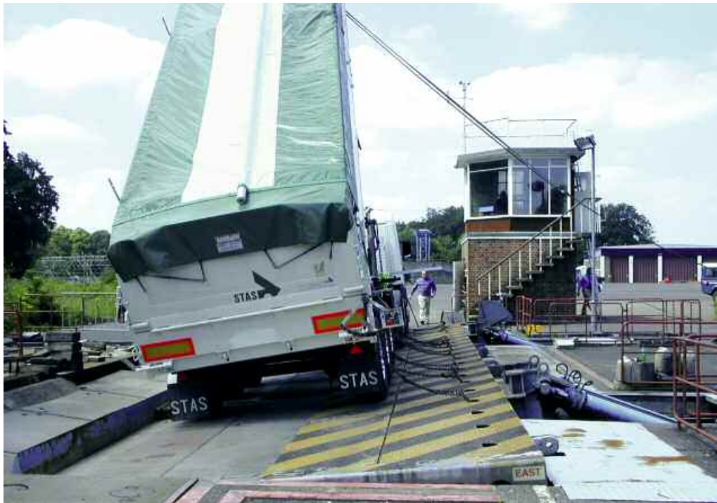
IRTE tipping stability test (STAS)
