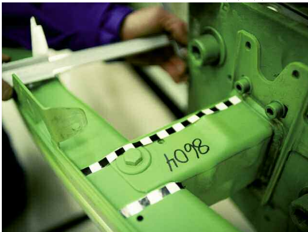
Aluminium bumper system prepared for crash test
