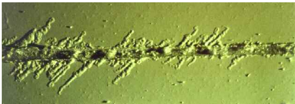
Filiform corrosion coming from defect in paint
