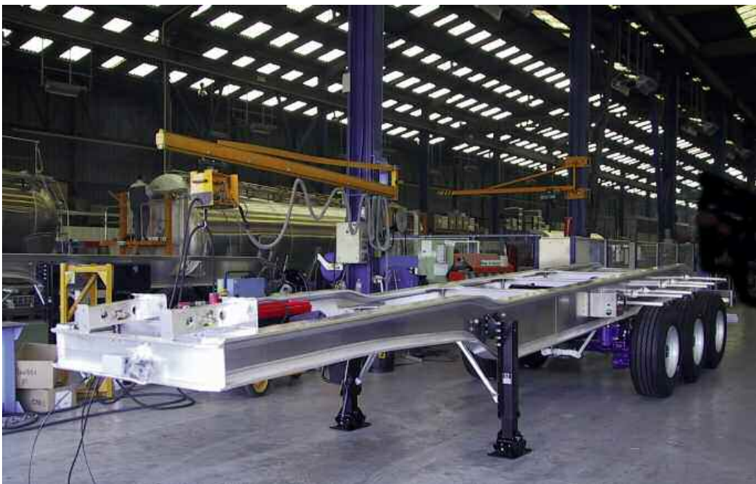
Chassis for aluminium tipper (Benalu)
