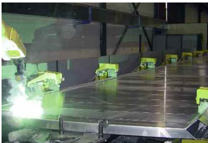
Welding of side panels for tippers (Menci)
