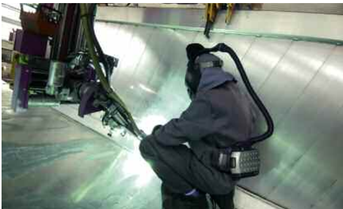
Welding of tipper body (SCHMITZ)
