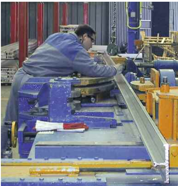
3-point press bending (Benalu)
