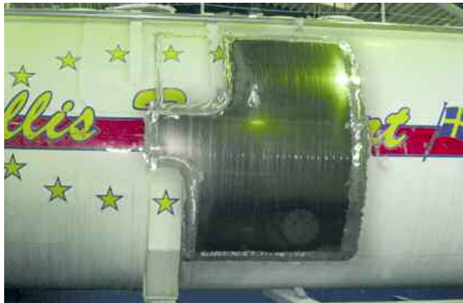
Outside view of a repaired aluminium tank (Feldbinder)
