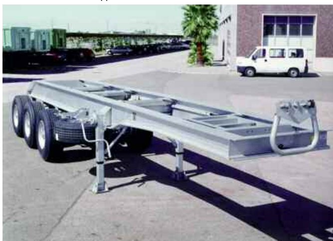
Chassis for aluminium tipper (Leciñena)
