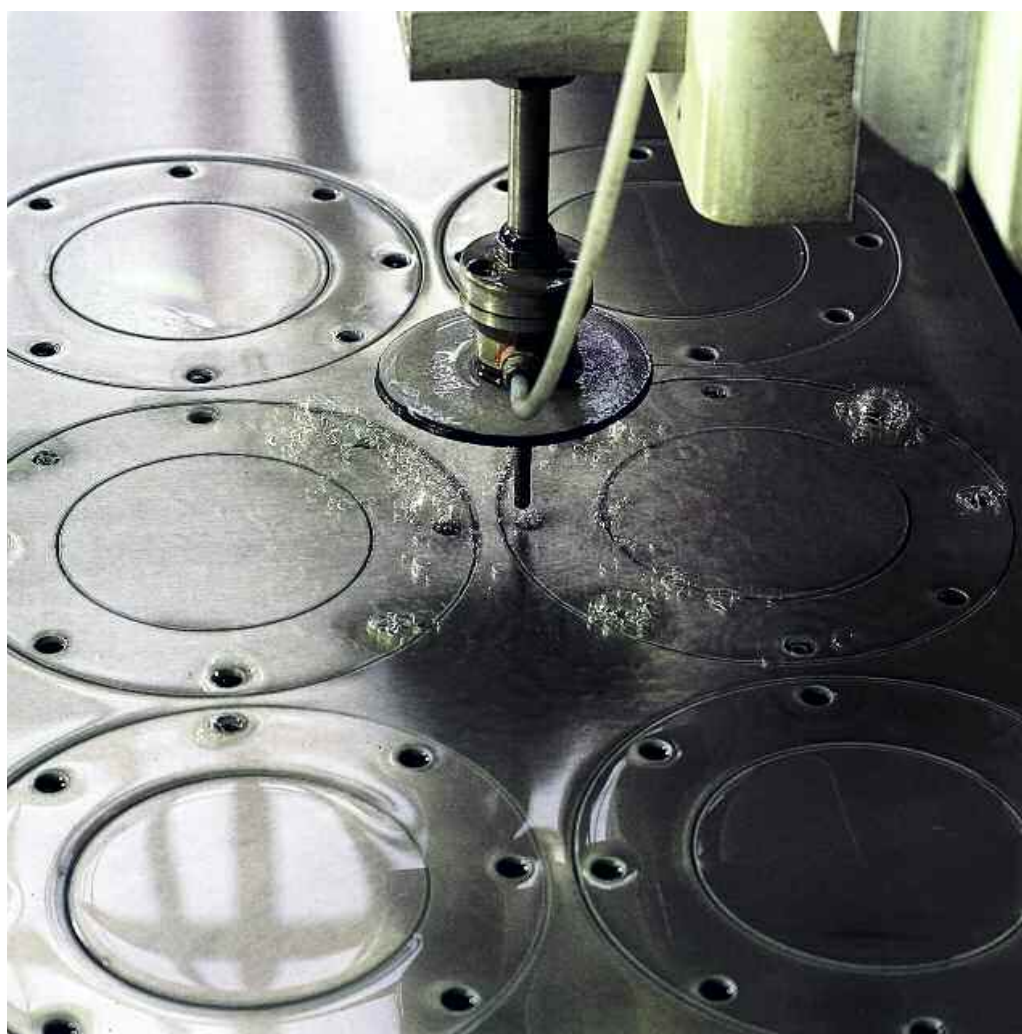
Water jet cutting (SAG)
