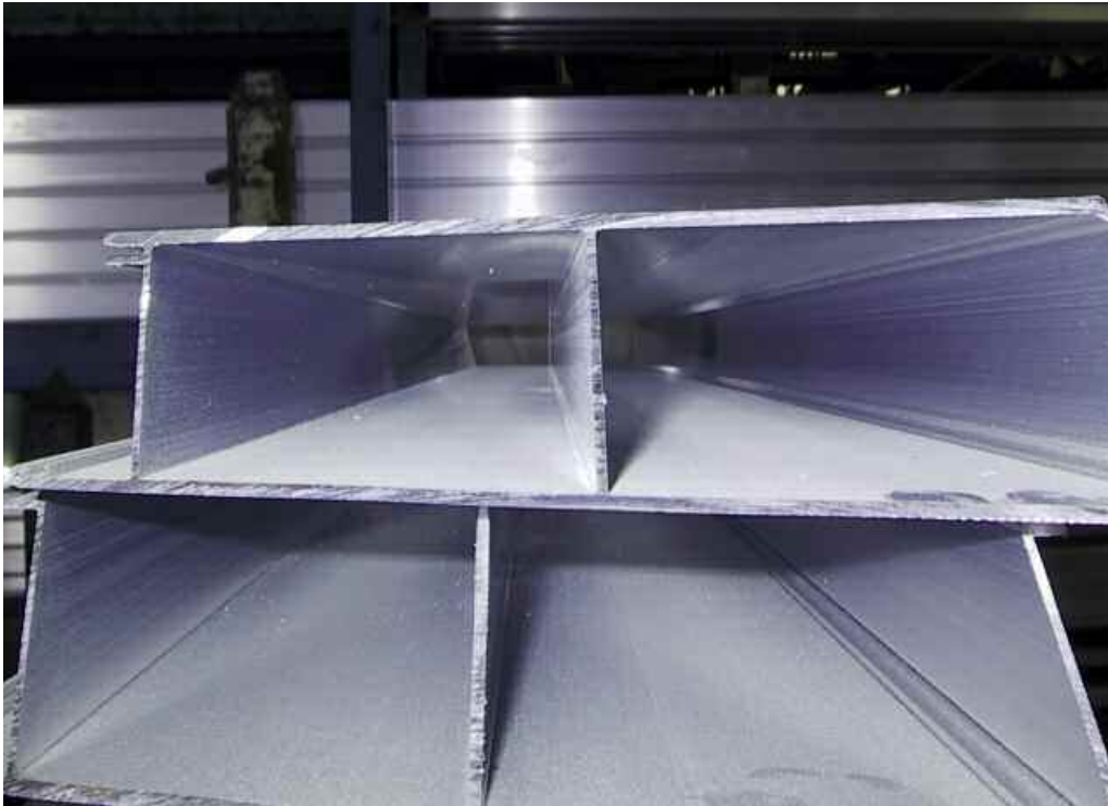
Double wall extruded boards for tippers
