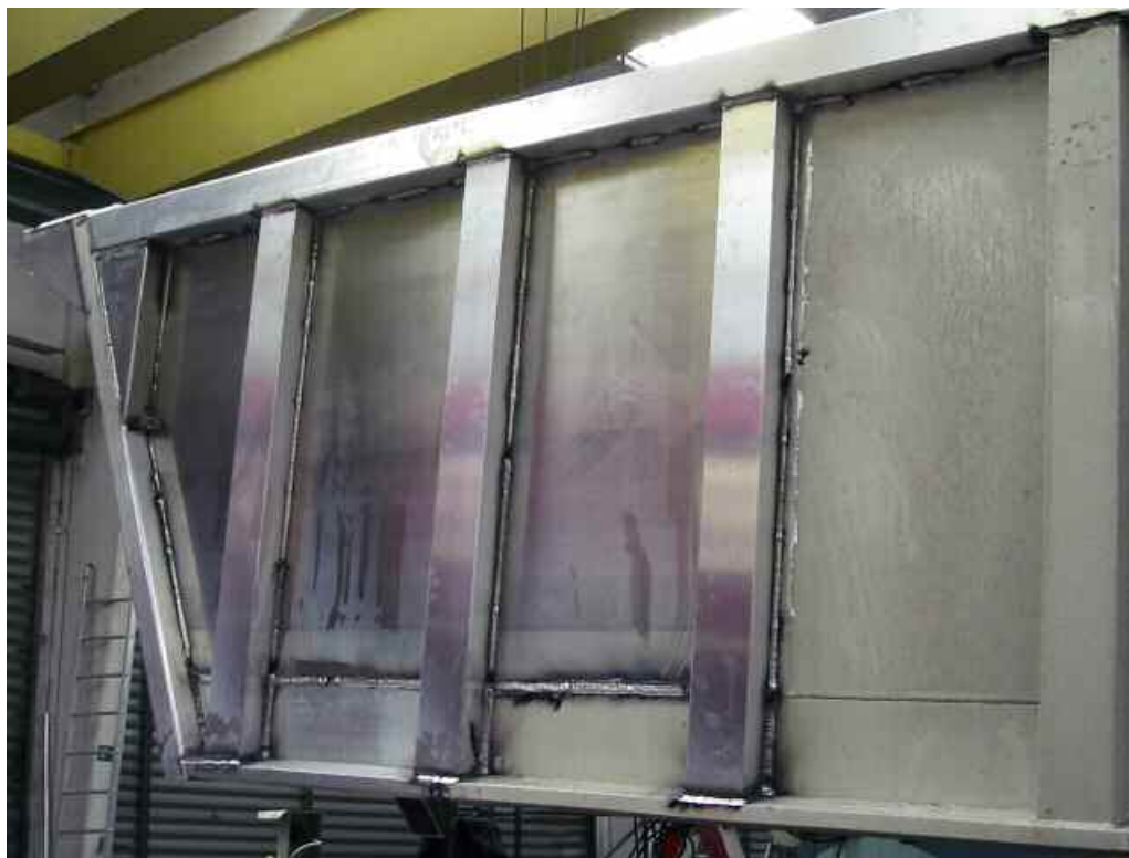
Repair of an aluminium tipper (Stas)
