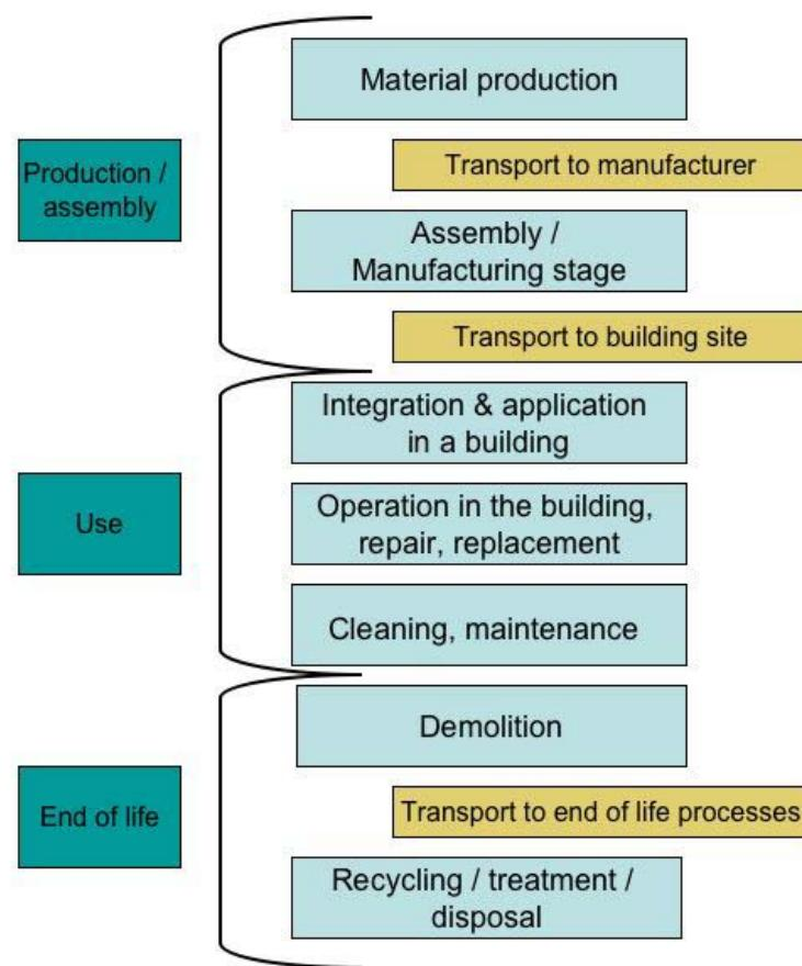
Fig 1: description of the Life Cycle stages of a building product
